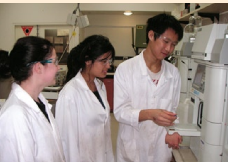
Parker Centre gold researcher Mrs Danielle Hewitt (far left) and two high school science students (who were participating in CSIRO's Student Research Scheme) getting ready to analyse a cyanide leach solution using the high performance liquid chromatography (HPLC) method for quantifying cyanide- and sulfur-containing species in solutions.
