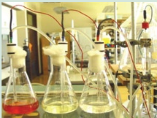
The "Biooxidation Process Water" project's apparatus for measuring the Eh (the solution potential) in multiple flasks of chemolithotrophic cell cultures. The common reference electrode is on the far right. The flasks from right to left show the progression of a batch culture as it converts approximately 100% iron(II) to around 100% iron(III) over 40 hours. Chemolithotrophic cells (used for bioleaching) catalyse biooxidation of sulfide minerals by oxidising iron(II) to iron(III) and creating a microcosm on the target sulfide mineral surface.
